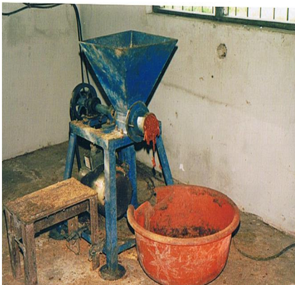
Figure 1b. Locally Fabricated electric pelleting machine
