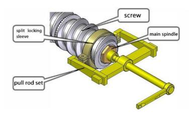
remove the first section of the screw. Besides, specific leads of the screw are also required by current removal tools. And it also takes a lot of labor and time to manually turn the screw lever, especially when some of the screws haven't been removed for years. For single screw extruders for aquafeed, however, the aforementioned method does not work out. See the structure of the screw for aquafeed extruders:
